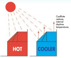
CoolKote protected conservatory roof reflects the sun's heat before it can be transmitted.
